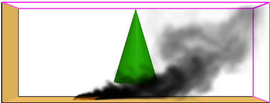
Figure 6.4 The geometry of the tree with an ignitor fire on the left with grass material on the ground.
